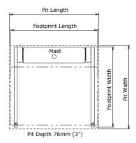
\*If a pit is used, recommended depth is 76mm (3"). Pit width and length include running clearances.
