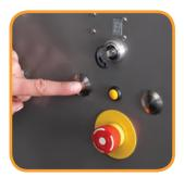
The easy to use control panel includes an emergency stop, a diagnostic display and a key lock.
